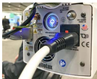
Remote cable connection to illuminator
