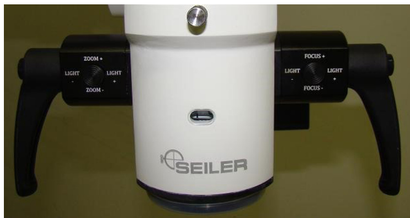
Figure 6: Joystick for adjusting zoom, light level and focus
